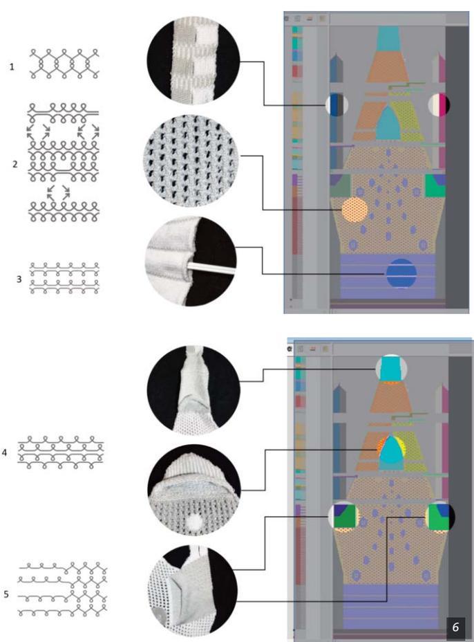
est tensile stress at the vertices. The interlock jersey structure at the knitted pocket carries sufficient tensile capacity to support the stress concentration at this end point.
