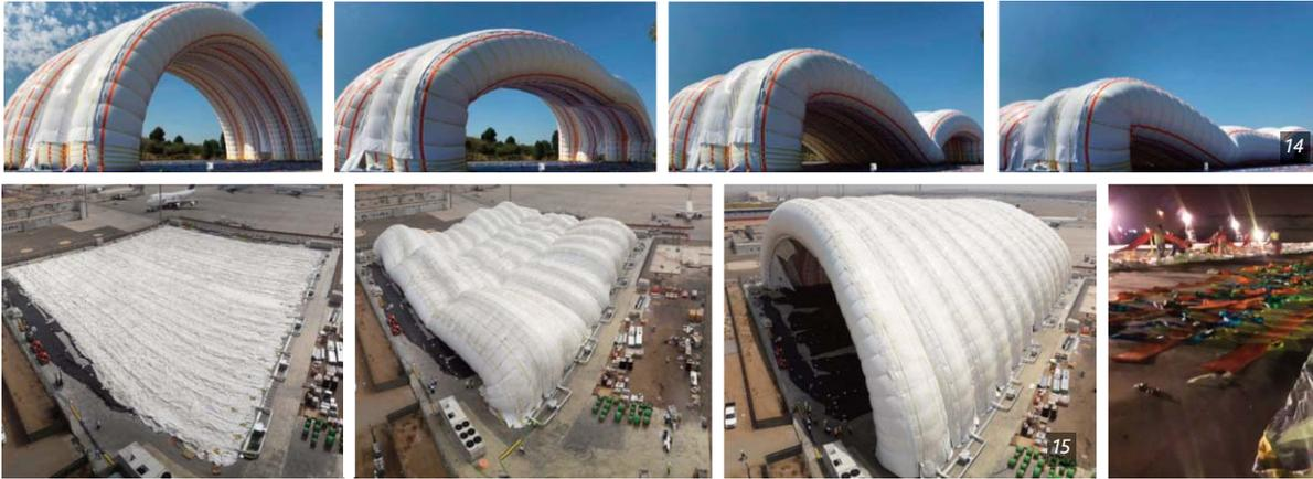
Figure 14. Deflation test showing initial state and after 15, 28 and 60min.
