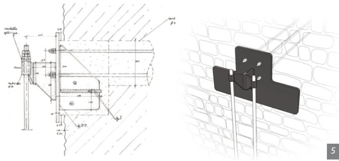
Figure 5. Anchor detail on the exterior side of the façade © Ney & Partners
