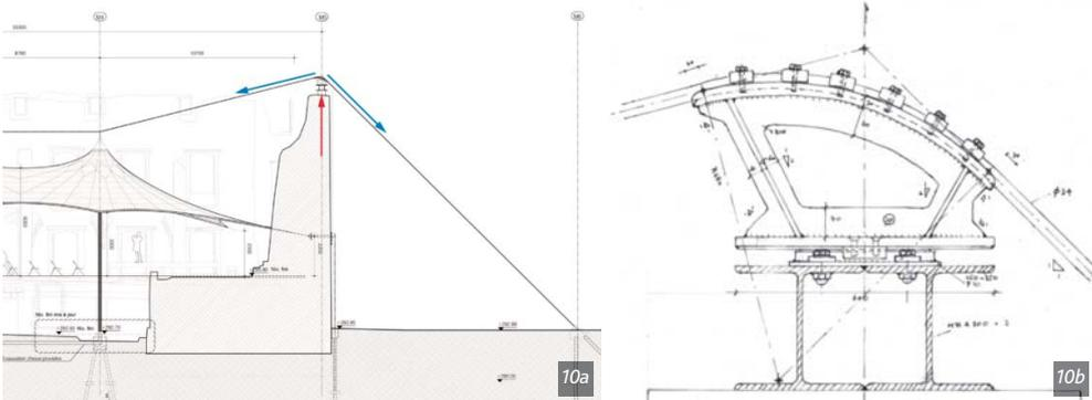
Figure 10a-b. Wall top deviation detail for the principal cable with sliding bearing. © Ney & Partners
