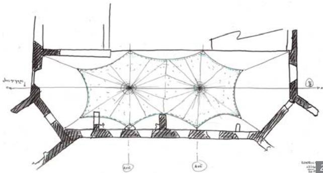
Figure 2. Sketch in the preliminary design illustrating the membrane and its fixation in the existing corps-de-logis © Ney & Partners
