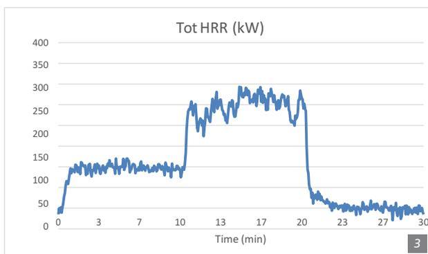
Figure 3. Heat release rate HRR during test, including burner heat output.
