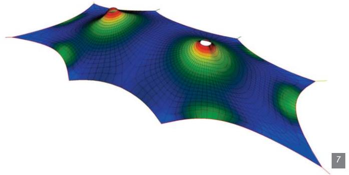
Figure 7. Stress concentration in the conical shape due to prestressing © Ney & Partners
