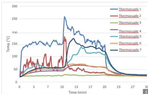
Figure 5. Gas temperatures in the door opening and temperatures on the external panel surfaces during the test. Position of thermocouples were according to table 2:
