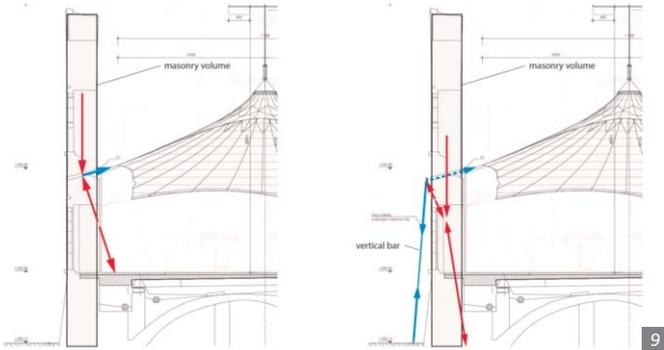
Figure 9. Strut-and-tie model of the reaction introduction: without reinforcement (left) and with external bars (right) © Ney & Partners
