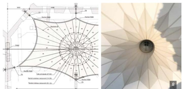
Figure 8. Cutting pattern and reinforcement layers © Ney & Partners
